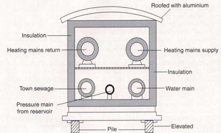
Figure 27 Cross-section of a utilidor. Source: Money (1980).
