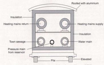
Figure 27 Cross-section of a utilidor. Source: Money (1980).
