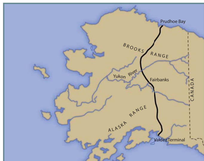
Alaska. Main physical features and location of pipeline. Permafrost occurs continuously in the Brooks Range and further north and to the west. It gradually thins out and occurs irregularly throughout the rest of the state, except for a small southern coastal strip where it is absent.
